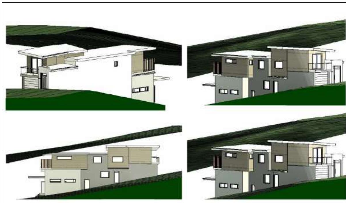
Figure 13 – Height Blanket Diagram
